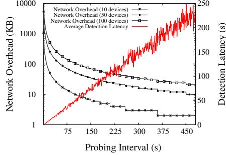
**Fig. 8: The effect of probing interval on network overhead and detection latency for SVELTE**
