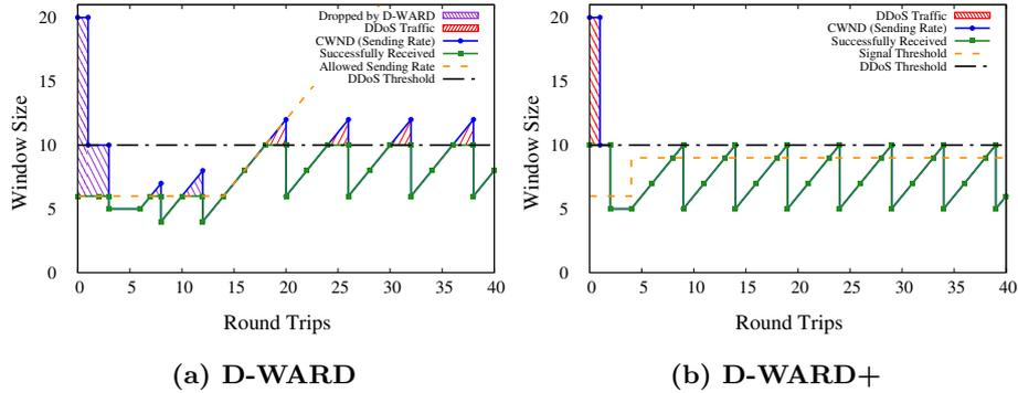
**Fig. 6: Behavior of a smart attacker under D-WARD and D-WARD+** large, a transient connection’s duration under D-WARD can be slightly faster (at most 3 seconds) than if it were under D-WARD+.
